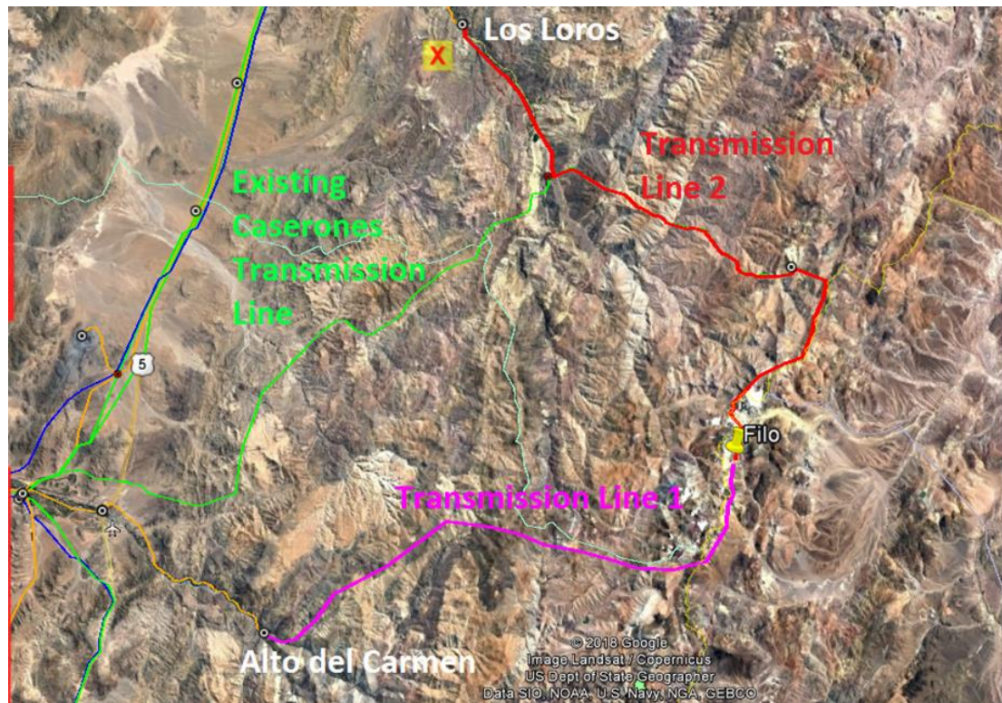
Figure 18-3: Transmission Line Route Options
